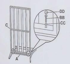
NOTE: Please ensure all the bolts are assembled correctly and use the allen driver (EE) to tighten. Do not fully tighten bolts/screws until all pieces are loosely assembled. Add corresponding plastic caps (DD) after final assembly finished.
